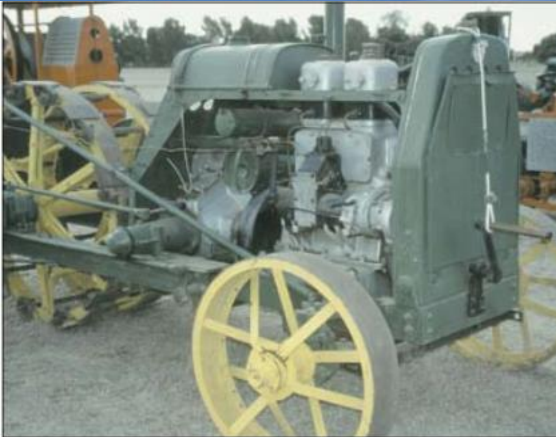
The two cylinder diesel engine can be clearly seen in this view of the off side of the Benz Sendling. (Photo IMU)
